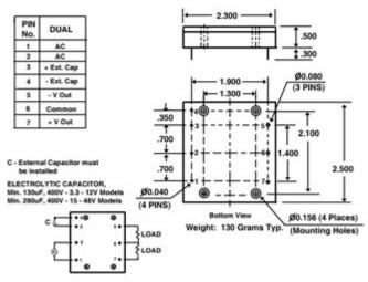
NOTE: The Recommended torque for mounting screws is 6 to 9 In-Lbs.
