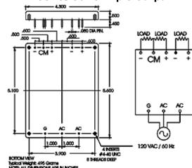
NOTE: The recommended torque for mounting screws is 3 to 5 In-Lbs.
