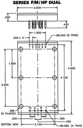
NOTE: The torque for mounting screws must be 6 to 9 In-Lbs.
