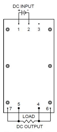
Notes: Pins 6 and 7 for remote sense, not on models with Vout > 48 V
