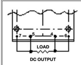
Note: Pins 6 and 7 are for models with output voltages up to and including 48 Volts. They are not on the higher voltage models (greater that 48 Volts)
