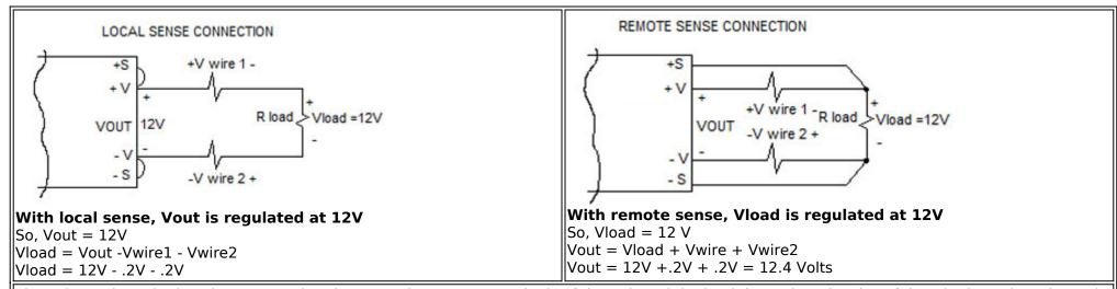
The voltage drops in the wires connecting the +V and -V output terminals of the unit and the load depend on the size of the wire )or pcboard trace) and the current flowing through them.
