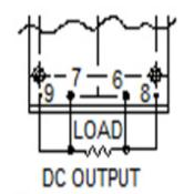
Pins 8 and 9 for sense must be connected.
